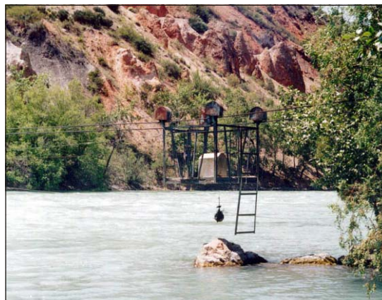
7.2. River gauging station on the Iskanderdarya River
