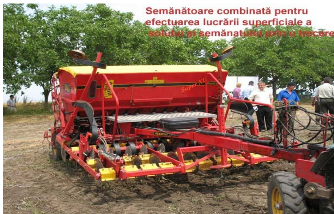
Fig.11. Agricultural machinery for the mini-till soil cultivation system
