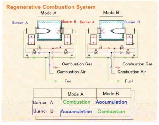
Figure A-8 Regenerative combustion system (Niga T, 2005)
