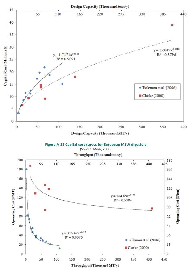
Figure A-14 Operating cost curves for European MSW digesters (Source: Mark, 2008)
