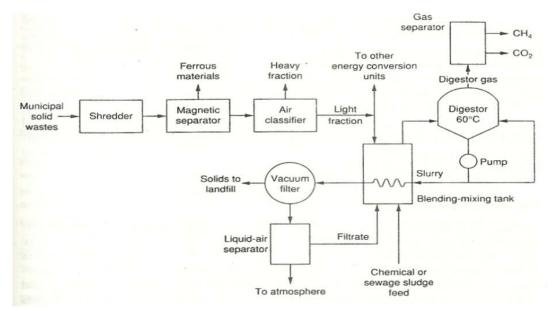
Figure A-12 Flow diagram for low solid anaerobic digestion process (Source: Tchobanoglous et al, 1993)
