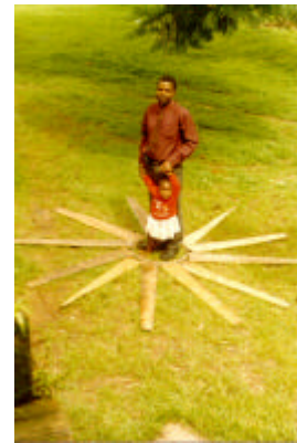
Fig 6.7 This is plywood, 12- bladed horizontal windmill under development at the Polytechnic in Blantyre suited for water pumping.
