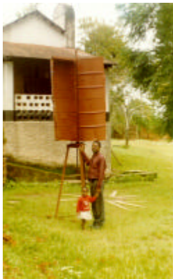
Fig 6.6. This a Savonius wind mill made out of semi-cylinders of steel oil drums. The design emphasizes the simplicity of the Savonius machine hence its possible adoption by the Malawian local communities.
