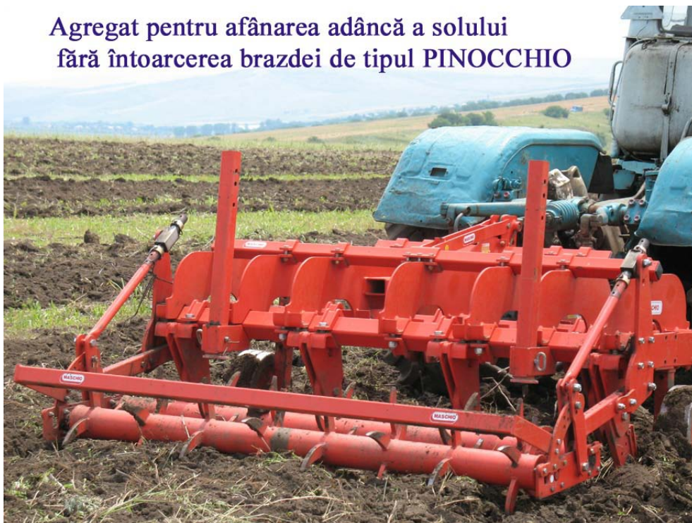
Fig.10. No-till soil loosening mechanisms
