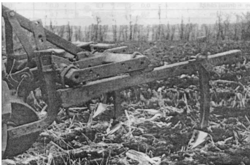
Fig.6. Ripper (on the basis of PRVH-2.5)
