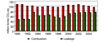
Fig. 3.4 Trends of emissions from combustion and leakage
