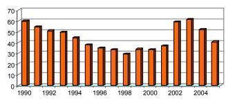
Fig. 7.4 Trend of CH<sub>4</sub> emission from industrial wastewaters
