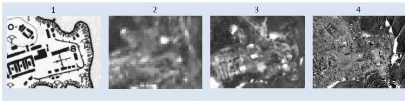
Figure 4: Comparison of all input data at a scale of 1 : 2,000 1: Topographic Map (scale 1:25,000); 2: SPOT-2 (resolution 10 m); 3: SPOT-4 (resolution 5 m); 4: WorldView-1 (resolution 0.5 m)
