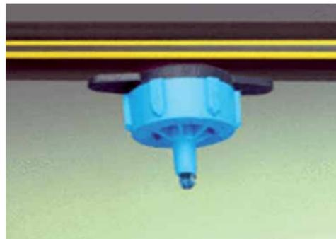
Figure 5.8b: Drip irrigation with black tubes.
