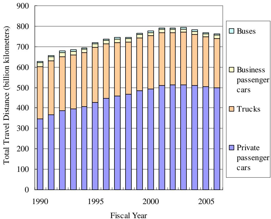
**Figure 1.18 Change in Vehicle Total Travel Distance**
