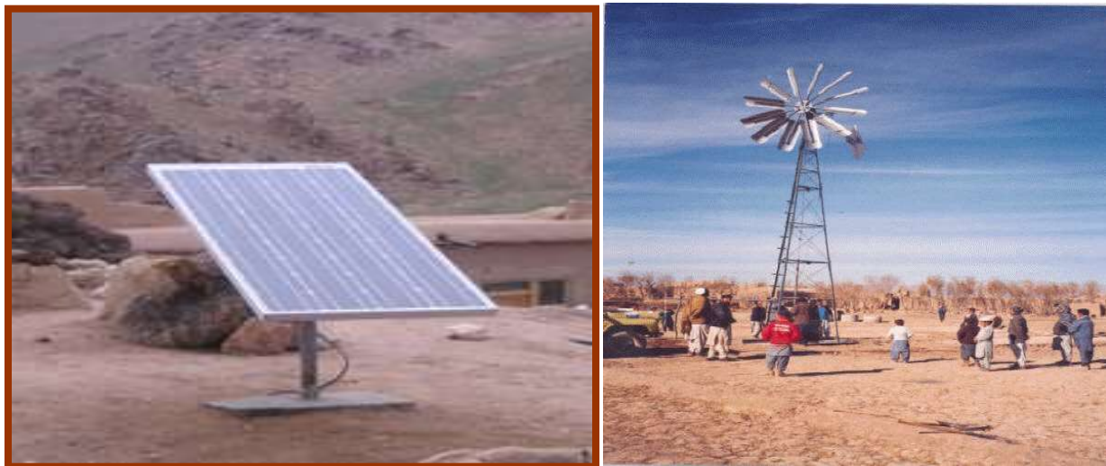
Solar system and wind mill in Afghanistan: Demonstration of 2 KW wind powered water pump in Herat.
