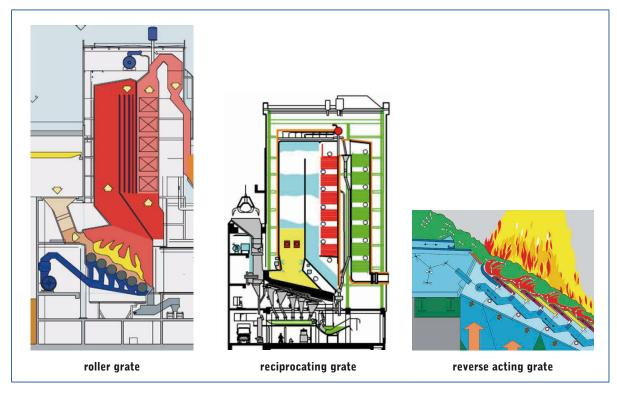
Figure 15: The three basic designs of grate furnaces: roller (left), reciprocating (central), reverse-acting grate (right)
