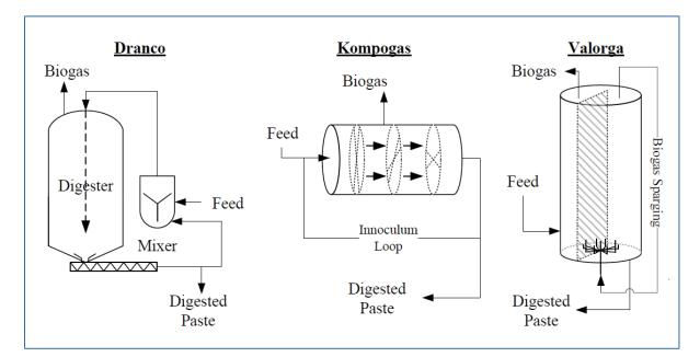
Figure 11: Solid-waste (dry) digester design: (a) Dranco, (b) Kompogas and (c) Valorga
