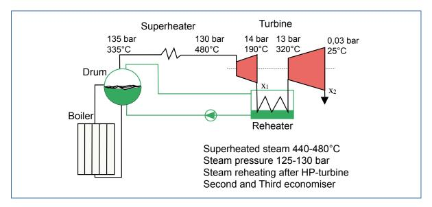
Figure 18: Intermediate steam reheating system
