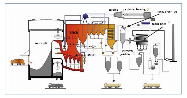
Figure 16: Stack gas treatment with SNCR, addition of activated carbon and fabric filter to remove NO<sub>v</sub>, dioxins and fly ashes
