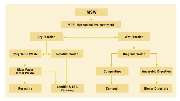
**Figure 1:** A typical dry-wet waste diversion model *MRF=Material Recovery Facility; LFG=Land Fill Gas*
