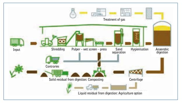
Figure 10: Process chain of a wet AD plant treating biowaste
