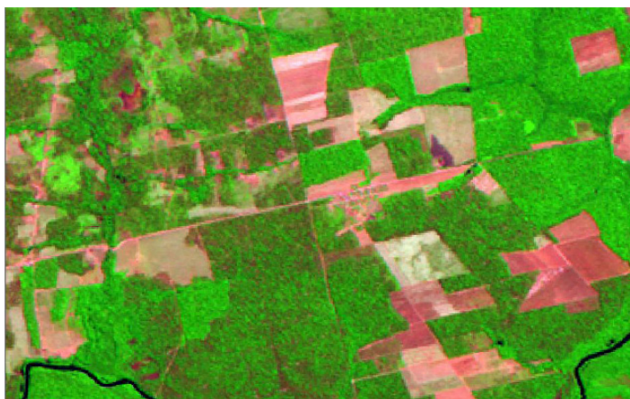
B) Color composition of LANDSAT data (TM3-Blue, TM4-Green, TM5-Red).
