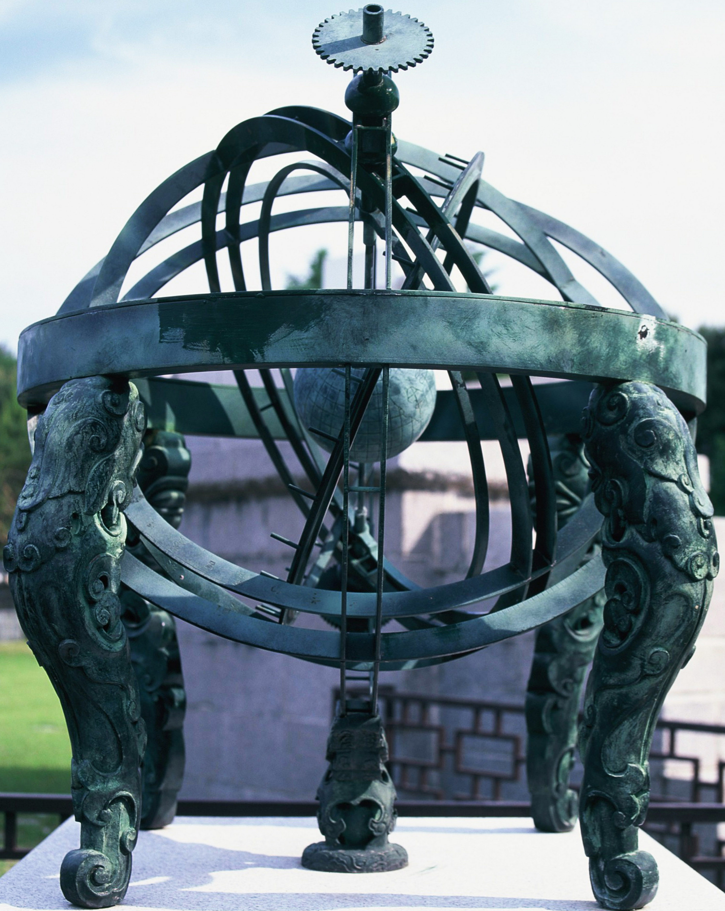
[Celestial Globe] An astronomical device to observe and measure the orbital movements of celestial objects
