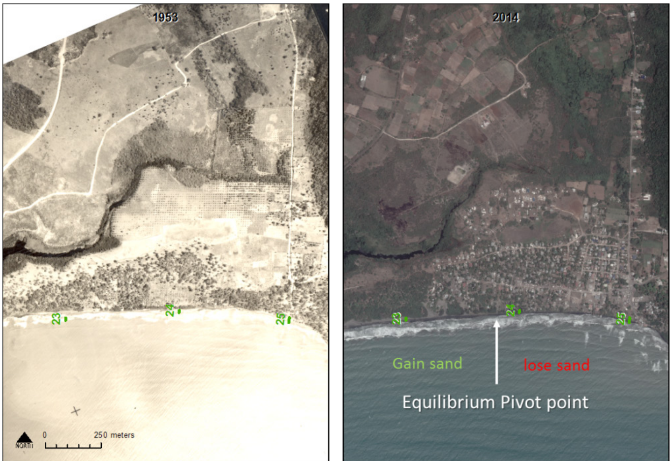
Figure 13: Comparison of 1953 aerial photo with 2014 satellite image. Location of profiles indicated on 2014 image
