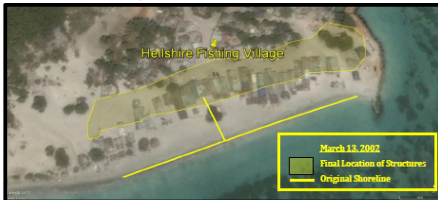
Satellite Imagery Time Series of Erosion/Sea Level Rise at Hellshire Beach March 3, 2002 – March 6, 2016 (The images for the period show progressive erosion of the shoreline)
