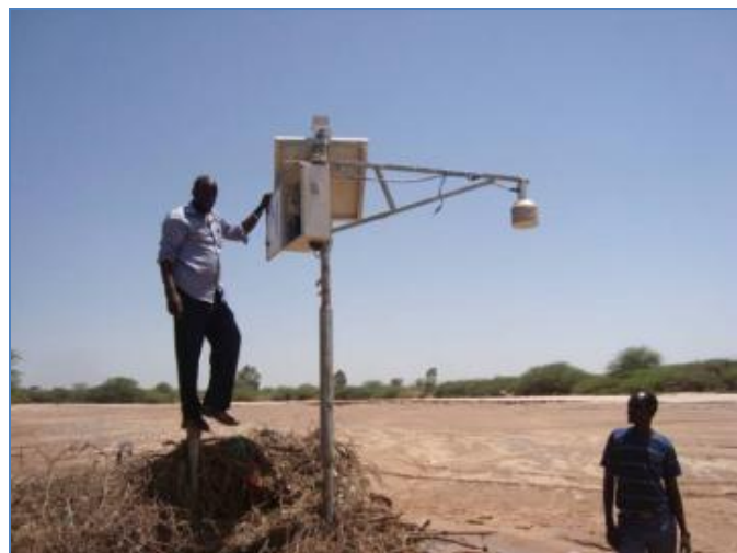
Figure 3-8 Installed automatic gauging station in Togga Waheen. Source: SWALIM, 2012.
