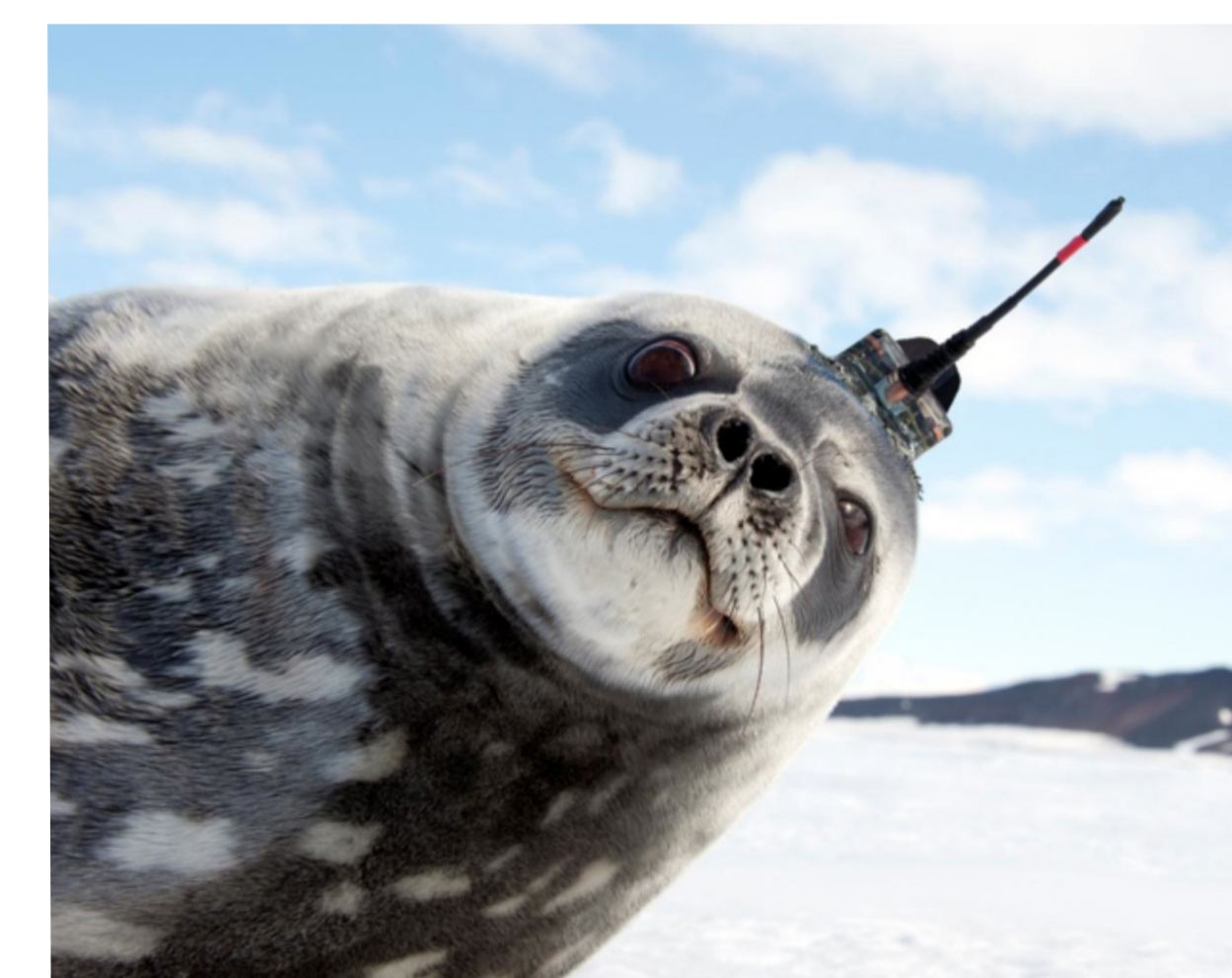
Small sensors on seals provide vital data on water column properties around the Antarctic coast & continental shelf.
