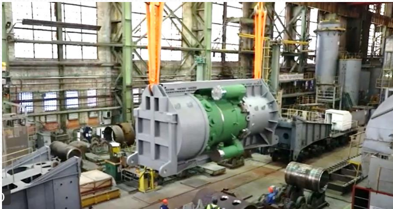
RITM-200 reactor at the factory
