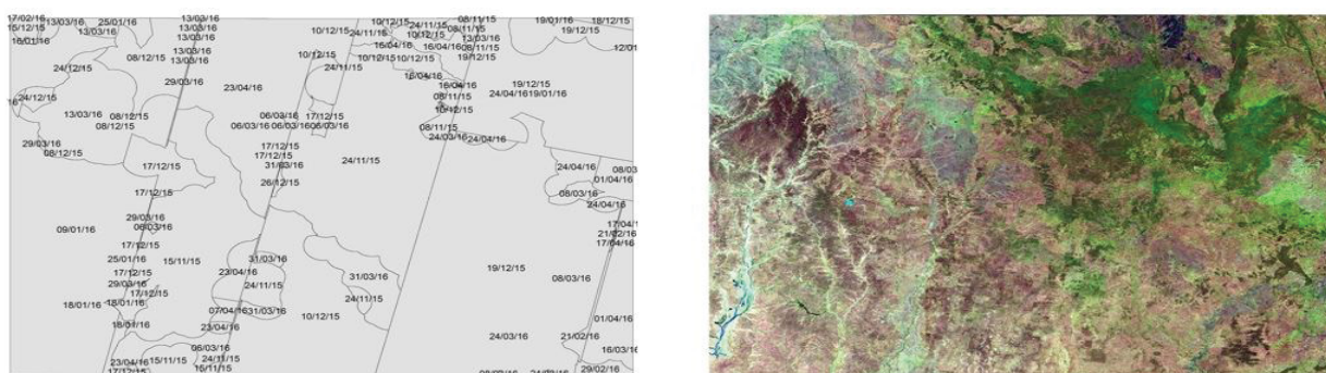
Figure A5.6.1.2 Image selection procedure, to create composite cloud free imagery mosaics
