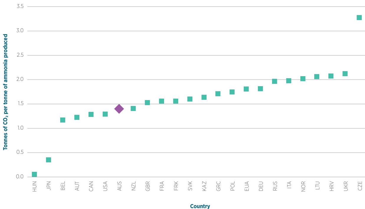
Figure 4.11 Ammonia implied emission factors for Annex I countries (2023 submission) and Australia (2024 submission), tonnes of CO 2 per tonne of ammonia produced
