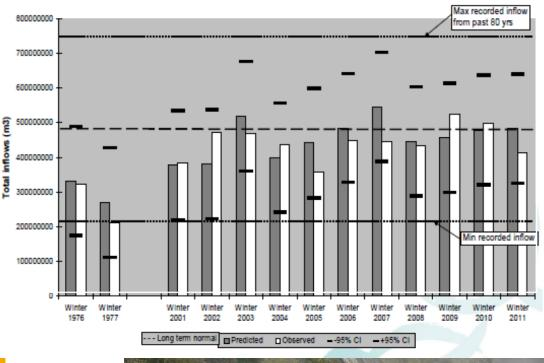
Reservoir operators can adjust water allocations to balance meeting hydropower generation targets with other priorities e.g. water supply, flood control
