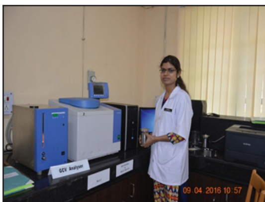
Figure 2.11: GCV determination of coal samples
