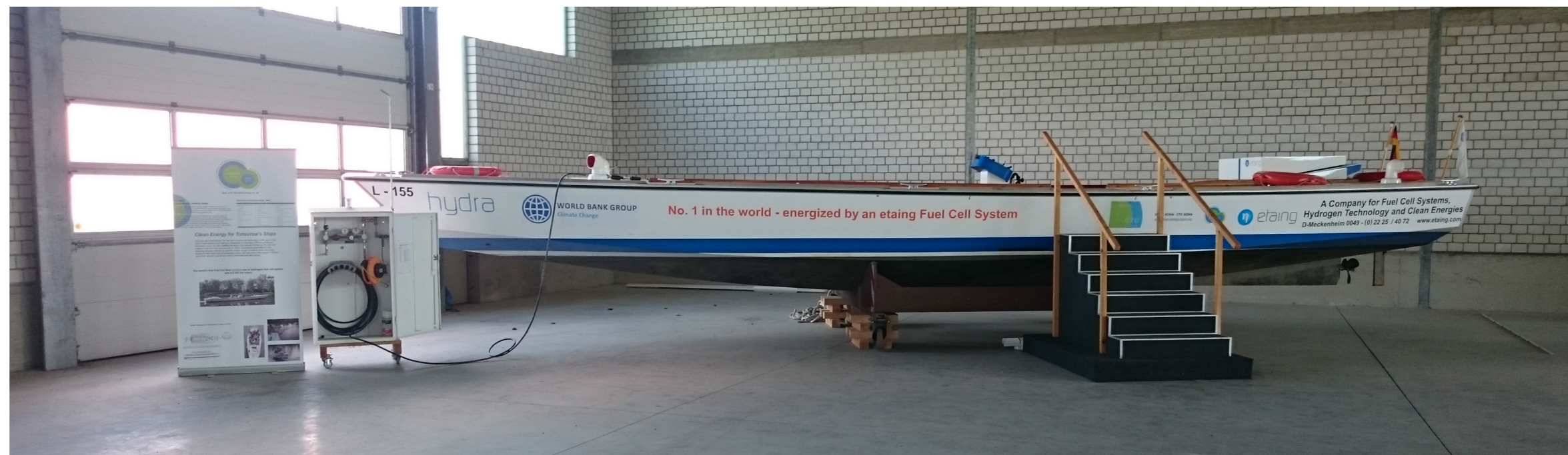
Hydra Boat. Electric mobility on the water by hydrogen gas/ fuel cells. A Project of ICEPS CTC BONN Technology Foundation
