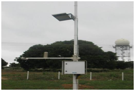
Figure 55: Automatic weather station in Accra
