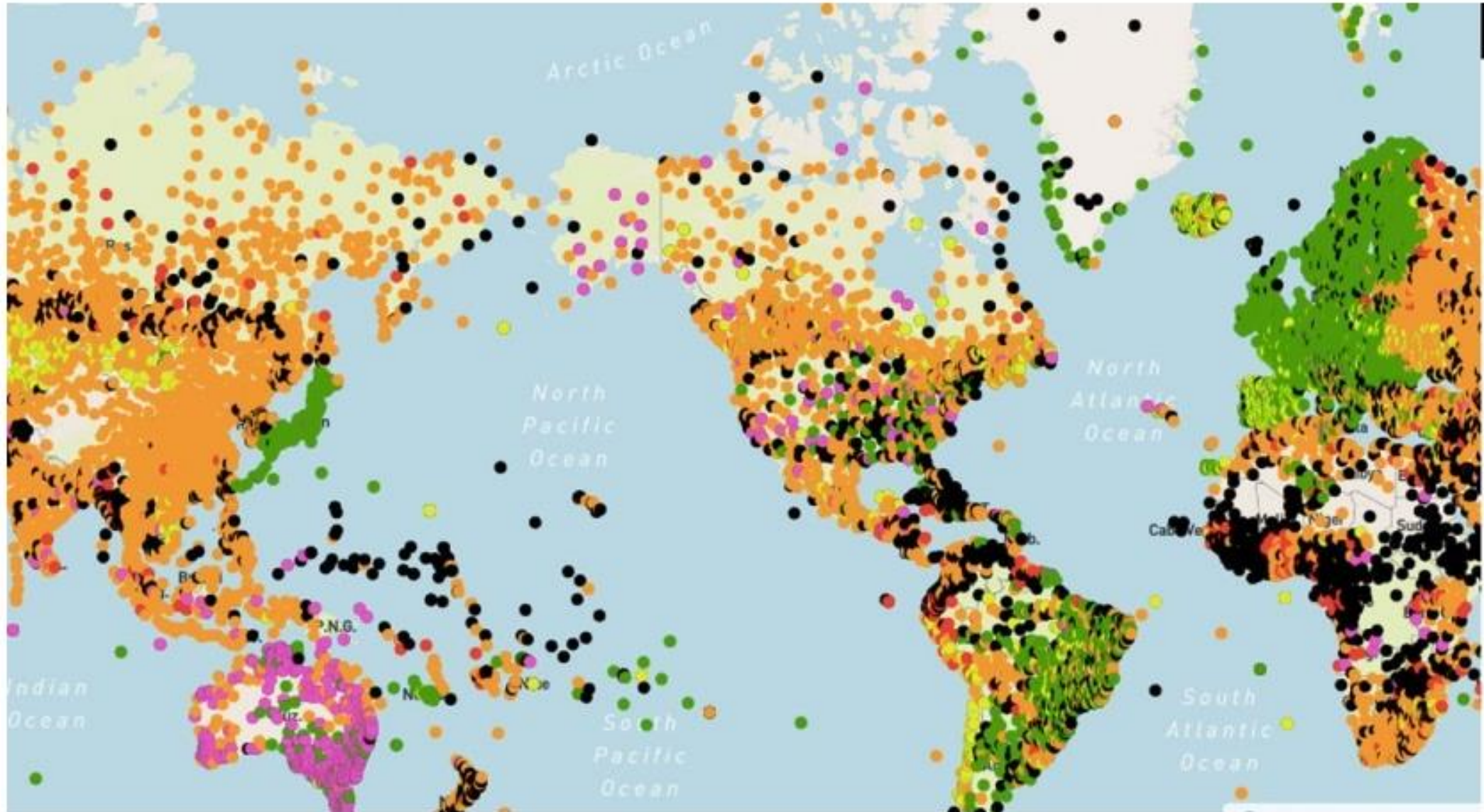
Surface land pressure observations reported by one or more global numerical weather prediction centres on June 27, 2018. Fully reporting stations shown in green, partly reporting stations in orange, minimally functioning stations in red, silent (non-reporting) stations in black.
