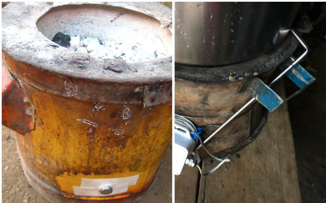
Figure. Example photos of SUM placement
