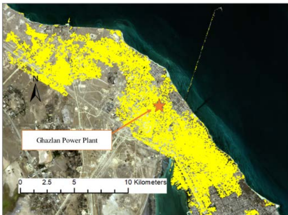
Figure 6.24 Flooded area when SLR at 2m
