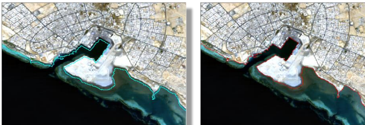
Figure 6.9: Geometric Correction Example Left (before correction); Right (after correction)
