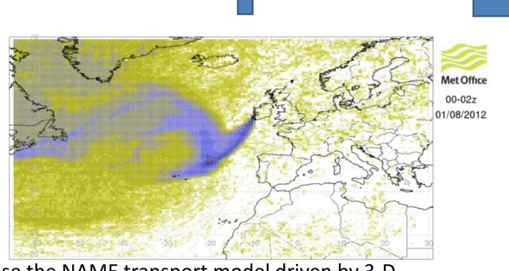
Use the NAME transport model driven by 3-D meteorology to understand the recent (3-4 weeks) history of the air arriving at measurement stations
