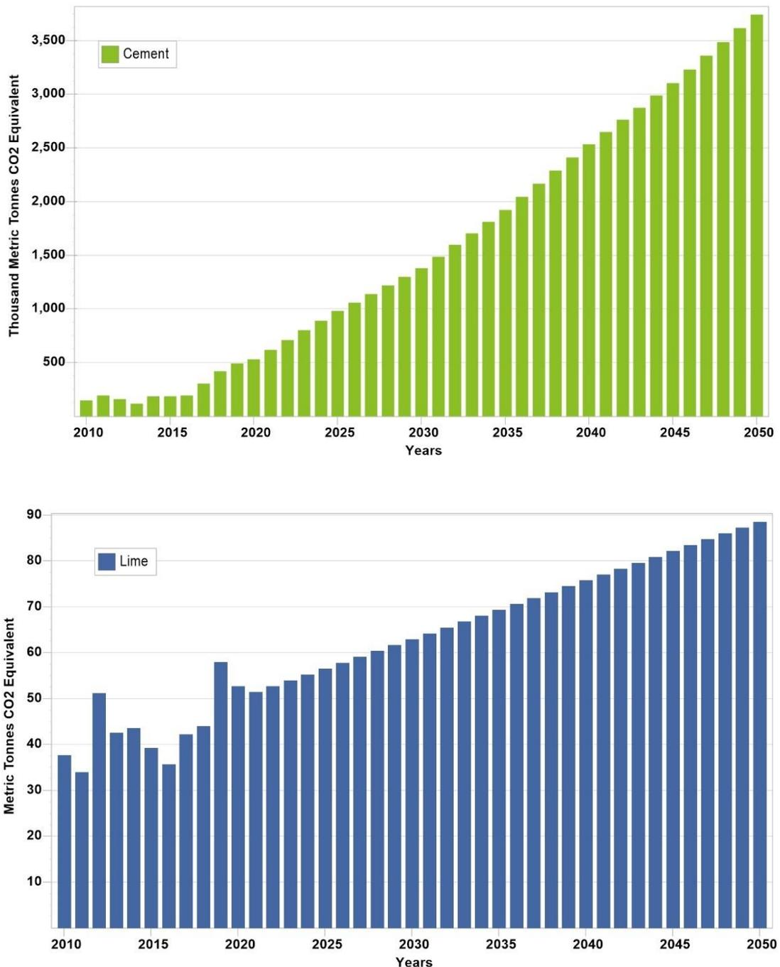
Figure 4-8: The baseline scenario for GHG emissions from the cement and lime industries (LEAP model)
