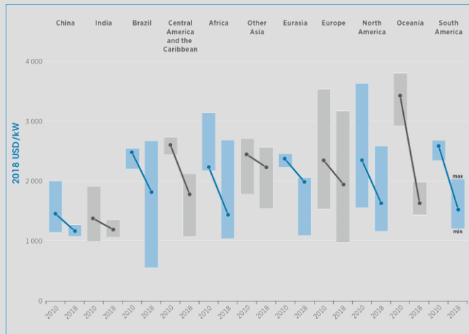
Figure 1.5 Total Installed cost ranges and weighted averages for onshore wind projects by country/region, 2010-2018
