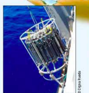
CTD sensor equipped with water sampling rosette deployed at the BATS station. © Woods Hole Oceanographic Institution
