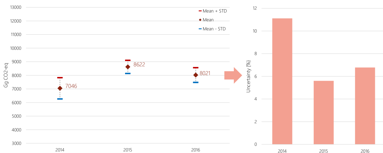
Figure 64. Total yearly emissions (and standard deviation) and total uncertainty for 2014, 2015 and 2016 using Error Propagation method
