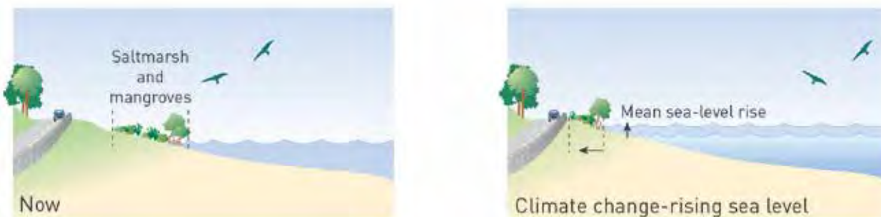
Figure 6.1: Coastal squeeze: built structures can prevent landward migration of intertidal ecosystems such as mangroves and saltmarshes.
