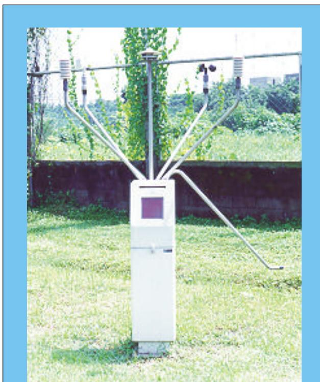
*An automatic weather station which has a solar panel that generates power for the system.*
