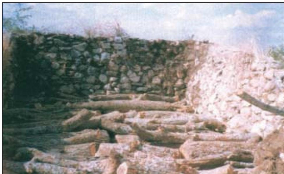
**Figure 2.5: Firewood logs in a Traditional Lime Kiln (Lirangwe, Blantyre)**
