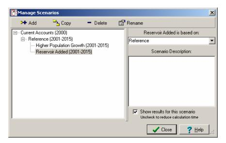
Then add a reservoir object on the Main River upstream of Big City, and name it "Main River Reservoir" Be sure to unclick the box where it asks if this object is active in Current Accounts.
