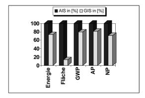
The use of GIS switchgears in the power grid studied lowers all the potential environmental impacts studied. The graph shows the relative environment impact potentials in the first year of use of the grid variants (dark bars=AIS variants, light bars=GIS variants).
