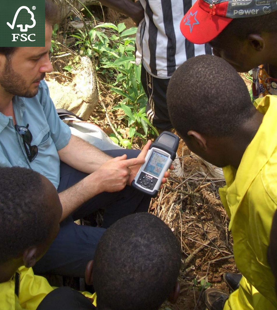
GPS handheld computer specially made for non-literate people and for forest use
