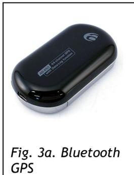
Many PDA's come with integrated GPS receivers. Using integrated receivers has a few drawbacks including reduced sensitivity of the receiver. Using an external receiver will overcome this problem giving the user the ability to move the GPS receiver away from obstruction. Commonly such receivers communicate with the PDA through a Bluetooth connection (figure 3a).
