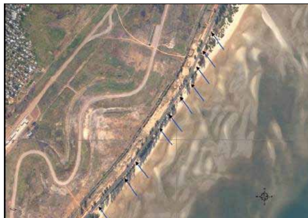
FIGURE 4: Marginal Avenue: Areas at risk of erosion from rising sea levels
