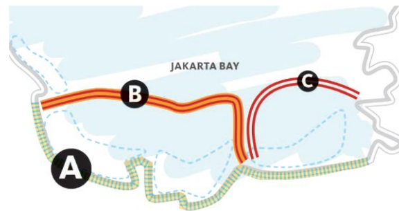
Figure 16 Three phases of the NCICD plan: A: embankment, B: sea wall west and waterfront city, C: sea wall east 474
