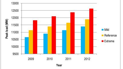
Figure 6.12 Peak loads for the period 2009-2012 taking into consideration the climatic effects, as projected by the Hellenic Transmission System Operator S.A.
