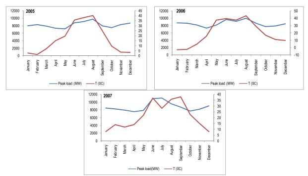
Figure 6.13 Monthly energy demand in MWH and temperature for the period 2005-2007, according to data provided by the Hellenic Transmission System Operator S.A.
