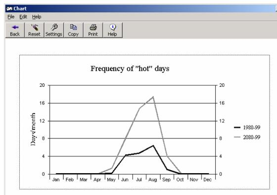
Figure 11.6 Monthly frequency of “hot” days (>25°C) at Blogsville downscaled using HadCM2 predictors under current (1960–1989) and future (2080–2099) forcing.
