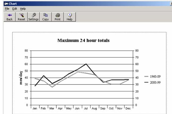
**Figure 11.9** Monthly maximum daily precipitation totals at Blogsville downscaled using HadCM2 predictors under current (1960–1989) and future (2080–2099) forcing.
