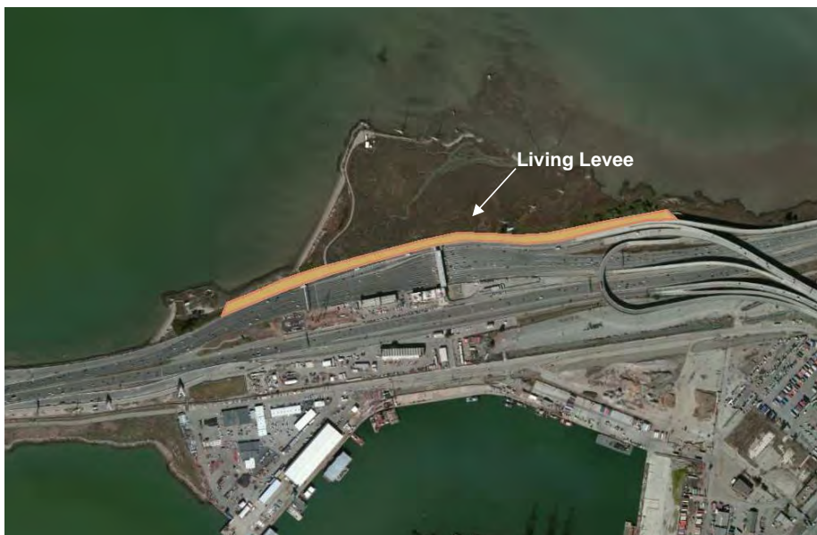
Figure 15: Aerial Graphic of Proposed Living Levee Along the San Francisco Bay Bridge Touchdown in California.
