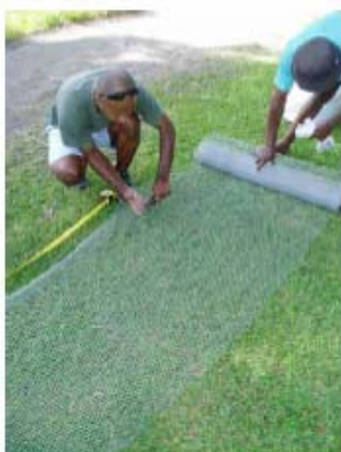
1. Cutting the chicken wire on the frame
